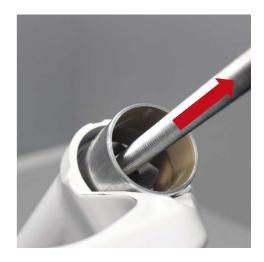
Lower slide bushing are thinner than upper slide bushings. Take lower slide bushing and orient its joint inside the fork. Drop it inside the casting. Do the same for the other lower slide bushing.
