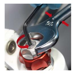
Use the 1.5mm HEX wrench to loosen the screw of the red knob. Clean the knob + screw. Store it.
