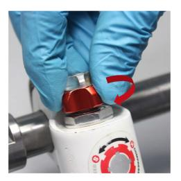
Loosen the air cartridge bolt. Clean the bolt and seals (x2). Store it.
