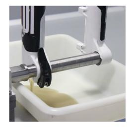
Loosen the oil cartridge cap.
