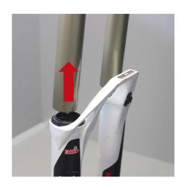
Place the tips of large retaining ring pliers into the eyelets of the retaining ring. Press firmly on the pliers and remove the retaining ring.
