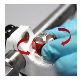
Rotate back the fork to its normal position. Take X ml\* of oil\*\* in a graduated pitcher. Unscrew the oil cartridge cap. Extend the fork at its maximum.
