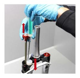
Screw the oil cartridge cap on the first thread.
