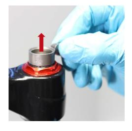
Connect air pump on the valve.
