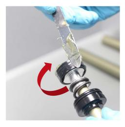
The groove should be full of grease!
