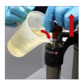
Screw by hand the oil cartridge cap until the stop. Compress and release slowly the fork 4-5 times.
