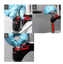
No torque – tighten to contact
