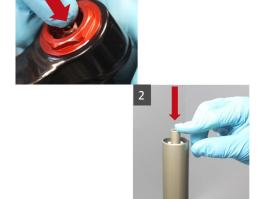
If your fork is TRC equipped and you cannot enter the air shaft: Place back the TRC button on the top of the fork.
