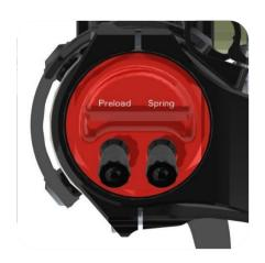
The air pressure is adjustied by the « SPRING » valve.
