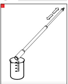
• Drain the closed cartridge in an oil pan
