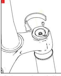
Slowly unscrew the cartridge bleed screw and allow the air to escape before replacing it
