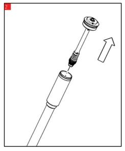
• Remove the compression block from the closed cartridge
