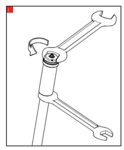
• Unlock the compression block of the hydraulic cartridge with two spanners 26 and 24
