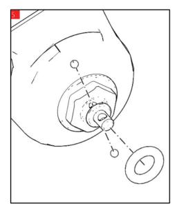
• Remove the O-ring from the hydraulic cartridge lower nut
