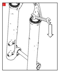
• Using a suitable open-end spanner, pry the lip of the seal to remove the scraper seals from the casting
