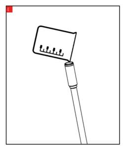
• Fill the closed cartridge with BOS BIOIL oil
