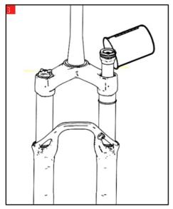
• Fill the air cartridge tube with BOS AMX6
