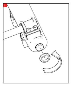
• Unscrew the lower nut of the air cartridge with a 21mm socket
