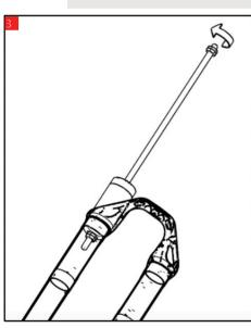
• Position the cylindrical body in the scraper seal housing
