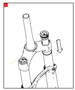
• Gently compress the fork to release the previously unscrewed air cartridge
