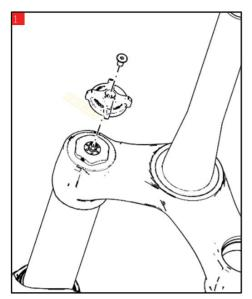
• Unscrew the holding compression knob screw with a 2.5 Allen key
