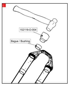
• Perform the same operation as for the lower ring but with the upper bushing tool
