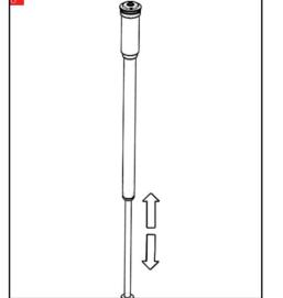
• Move the rod back and forth again to ensure that the closed cartridge is properly purged
