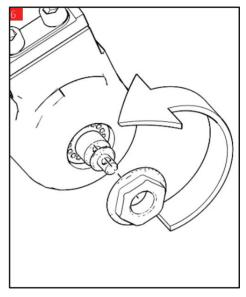
• Unscrew the lower hydraulic cartridge nut
