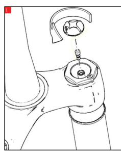
Unscrew the air cartridge top cap
