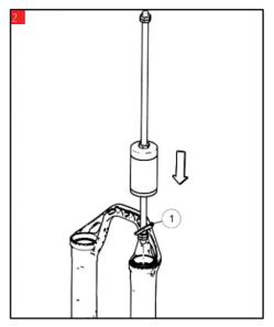
• Insert the guide ring removal tool into the casting
