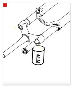
• Drain the content of your hydraulic tube in an oil pan
