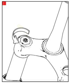
• Unscrew the hydraulic cartridge with a 26mm socket
