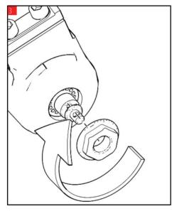
• Tighten the lower cartridge nut to a torque of 10Nm
