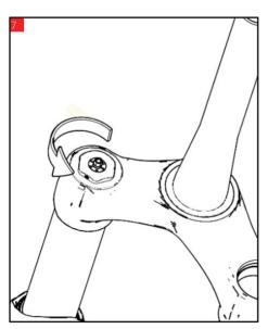
• Tighten the hydraulic cartridge in the fork tube
