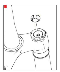
• Screw the top cap of the air cartridge back on by hand
