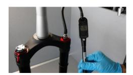
Apply grease by hand on the air cartridge bolt and O-rings. Screw the bolt in the shaft with a torque wrench + 5mm HEX socket. Increase pressure until the user pressure has been reached.
