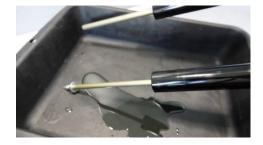
Firstly, remove retaining ring screw then Place the tips of large retaining ring pliers into the eyelets of the retaining ring.
