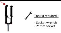
Disassemble the oil cartridge from the chassis Loosen the cartridge from the crown. Remove slowly the cartridge from the chassis, clean it.
