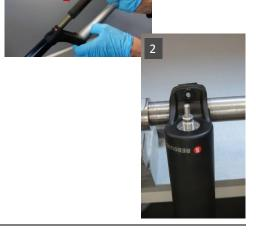
Degrease and clean the bottom of the oil cartridge (seal and thread). Degrease and clean the bottom of the casting Insert the oil cartridge in the fork. Screw the oil cartridge nut on the first threads.
