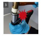
Change the upper O-ring in the floating piston. Change the main piston O-ring.
