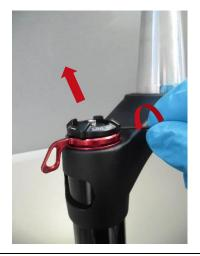
Use 1.5mm HEX wrench to loosen the two screws of the platform adjustment. Clean the platform adjustment + screw (x2). Store it.
