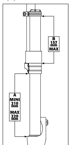
When installing the wheel with a properly inflated tyre check to make sure that the forks achieve minimum tyre clearance. Simply measure the distance from the top of the leg (lower part of the seal) to the outer of the lower crown, it has to be between 210mm to 220mm (A).
