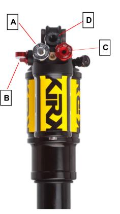
during your run. You risk setting your shock for 3% of the course and losing efficiency on the other 97%. If your shock doesn't get full travel, soften the high-speed compression by turning the knob counter-clockwise.
